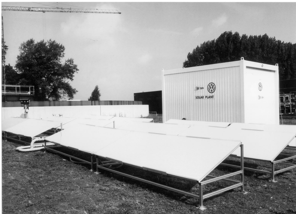
Fig. 14. View on the pilot plant for the solar photocatalytic treatment of a biologically pretreated wastewater installed in Wolfsburg, Germany (Photo: Volkswagen AG).
